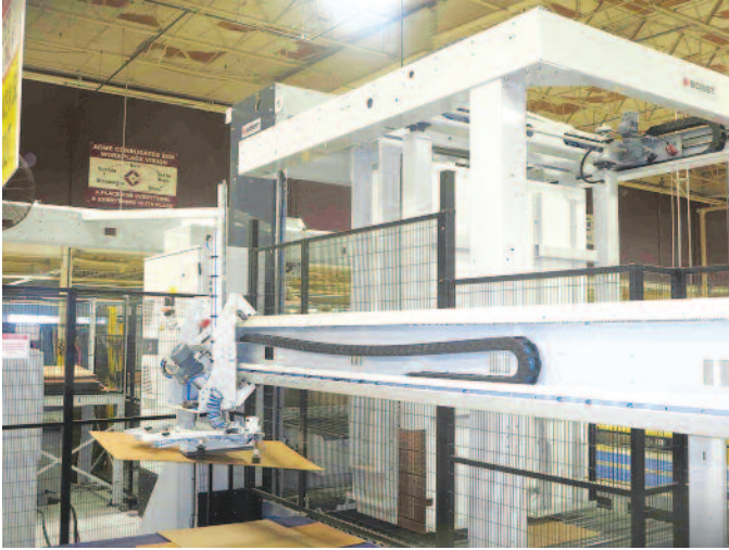
Two of Acme's four machines are full-line Bobst, which include prefeeder, flexo and palletizer.
