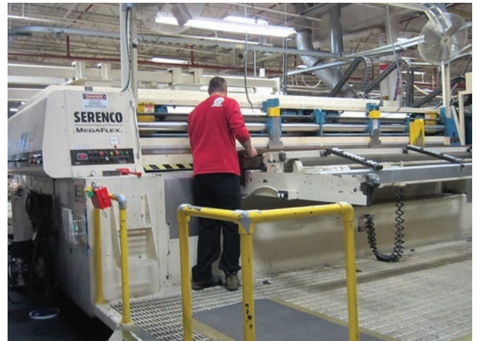
Acme’s Serenco jumbo flexo, which was retrofitted with an Absolute Engineering chamber, was also repositioned in the plant to provide for an enhanced flow of finished goods.
