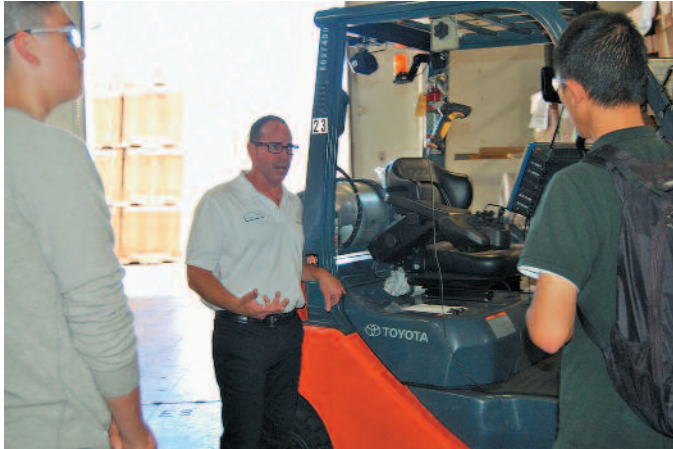
21st century technology covers all aspects of boxmaking, as Bay Cities' COO Brett Kirkpatrick shows how computers fitted on forklift trucks keep track of finished goods inventory.
